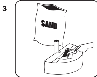
3 Using a scoop or funnel, fill the SOLO™ weight bag with approximately 50lbs/22.5kg of clean dry sand.
