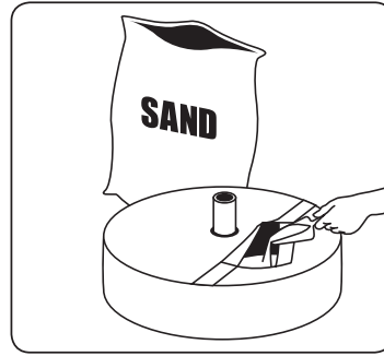
Pull the velcro tab on the top of the Gravipod™, and using a hand shovel or funnel fill with play sand, to your desired weight, up to 85lbs/38.5kg.
